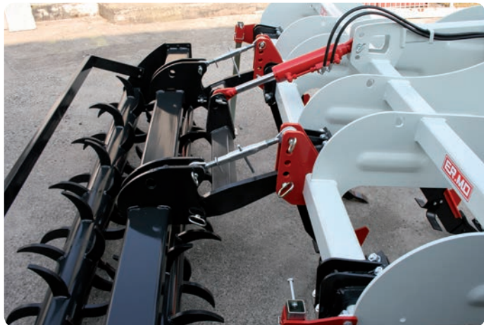
Detail of the double rear spike roller with hydraulic depth adjustment.
